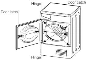
The door of your dryer is reversible and can easily be changed. Exchange diagonally hinge brackets and blanking screws. Exchange door latch and catch with their opposite blanking plates (*see diagram above*).
